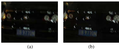
Fig. 20. A failure example by the proposed algorithm on the blurred image with numerous outliers. (a) Blurred input. (b) Deblurred output.
