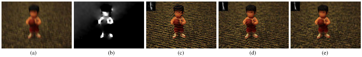
Fig. 14. A real captured image with blurry background textures. Our method generates a clear image with fewer artifacts. (a) Blurred image. (b) f_W(\delta B) . (c) Cho and Lee [3]. (d) Xu et al. [11]. (e) Ours.
